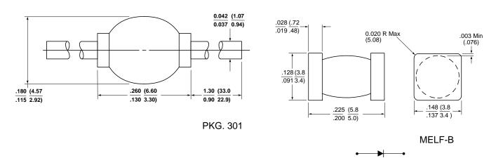
Note: The cathode side is marked with a dark colored band on one side of the diode body.
