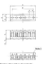
Note1: Contact No. indicates all number of contacts. Note2: Do not clean the cable with heat nor trichloroethane. Contact insertion view
