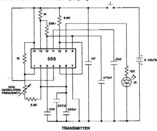
\*Ground Pin 6 and adjust for 40 kHz  $\pm$  2 kHz from Pin 9 with parallel/series resistance.
