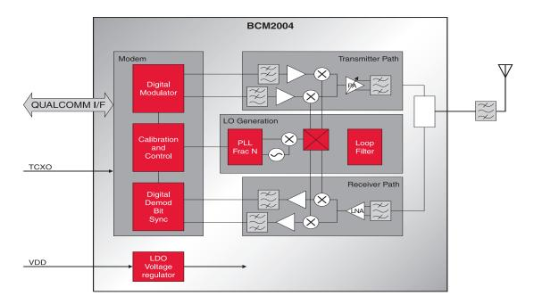
The **BCM2004** Bluetooth transceiver is an integrated radio transceiver that is optimized for use in QUALCOMM MSM-based wireless systems. The transceiver is Bluetooth 1.1, 1.2, and 2.0 compliant and is designed to enable simultaneous operation with any of the radios options, including GPS, WCDMA, CDMA, and GSM/GPRS.
