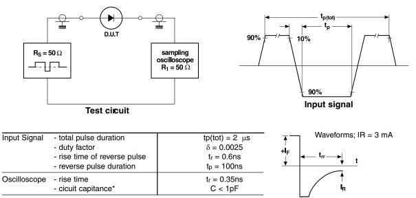
\*C = oscilloscope input capactitance + parasitic capacitance
