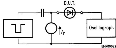
Pulse generator:  $t_p = 5 \mu\text{s}, D = 0.05$
