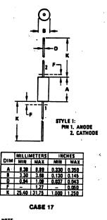
NOTE: 1. LEAD DIAMETER & FINISH NOT CONTROLLED WITHIN DIM "F"
