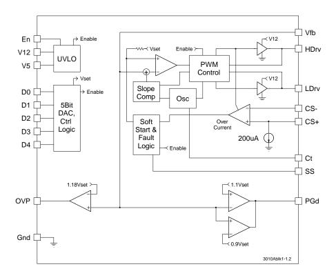
Figure 1 - Simplified block diagram of the US3010/3010A.
