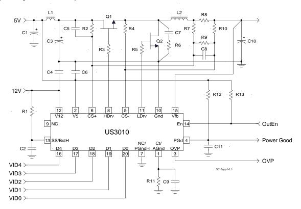
Figure 2- Typical application of US3010/3010A in an on board DC-DC converter providing the Core supply for the Pentium II microprocessor.
