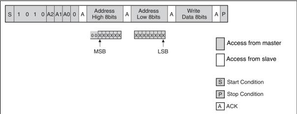
Note: In the MB85RC128, input "00" as the upper 2 bits of the MSB.
