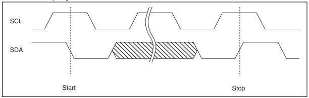
Note: The FRAM device does not need the programming wait time (twc) after issuing the Stop Condition during the write operation.
