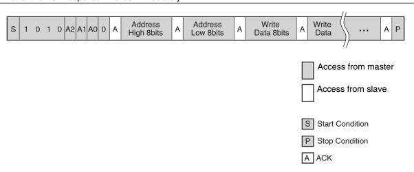
Note: It is not necessary to take a period for internal write programming cycles from the buffer to the memory after the stop condition is generated.
