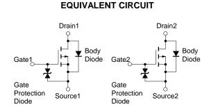
Remark The diode connected between the gate and source of the transistor serves as a protector against ESD. When this device actually used, an additional protection circuit is externally required if a voltage exceeding the rated voltage may be applied to this device.
