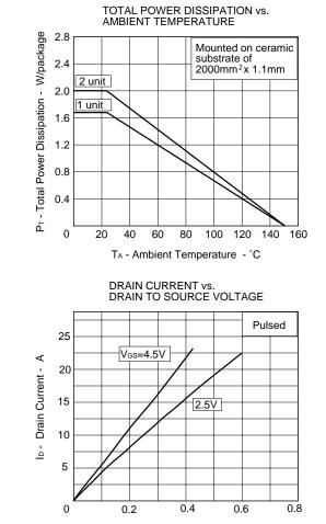
VDS - Drain to Source Voltage - V
