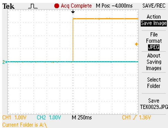
Figure 6: Startup Pop-Noise with PUNK
