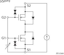
Test Circuit 7 t<sub>d</sub>(on), t<sub>r</sub>, t<sub>d</sub>(off), t<sub>f</sub>
