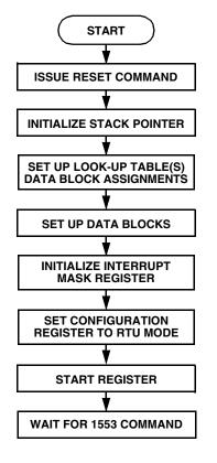
Figure 19 – RTU Initialization
