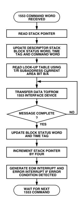
Figure 22 – RTU Message Transfer Operation
