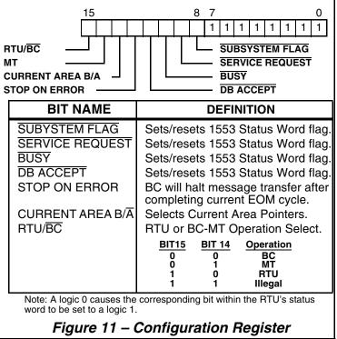
**REGISTER.** This write-only register is used to reset the CT2553 and to start the BC and MT operations, as illustrated in
