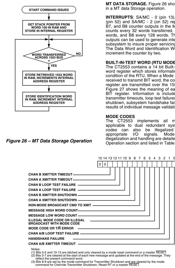
MT DATA STORAGE. Figure 26 shows the steps in a MT data Storage operation.
