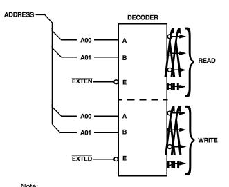
Note: A02 of the CT2553 must be set to logic 1 to operate with external registers.
