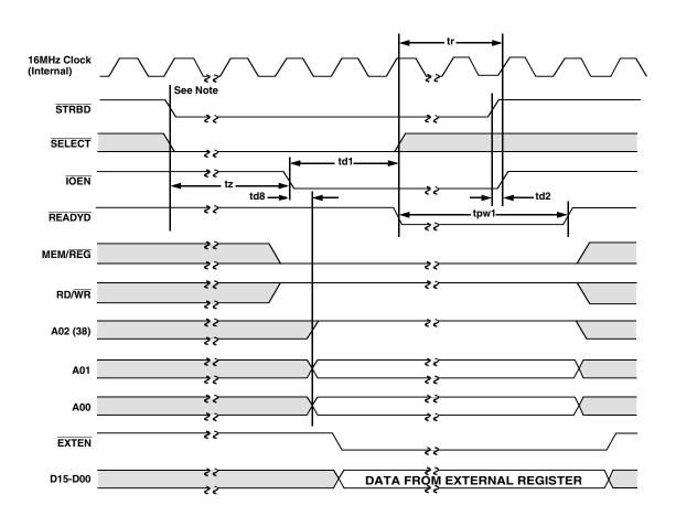
NOTE: STRBD to IOEN (low) delay is two clock cycles. If contention occurs, delay is two clock cycles following release of bus.
