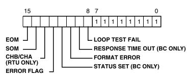
Note: In BC <u>operation</u>, the CT2553 always writes the BSW to RAM with Bit-13. CHB/CHA toggles as per the message control word setting.
