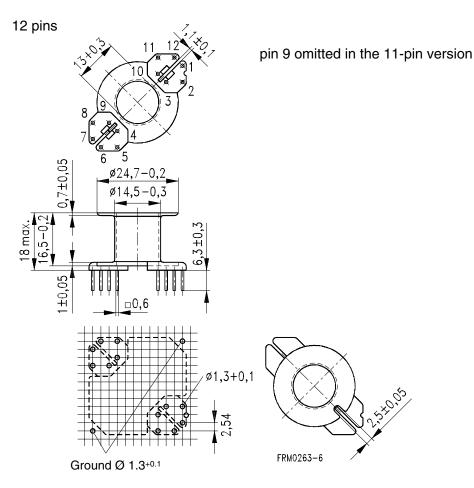
Hole arrangement View in mounting direction
