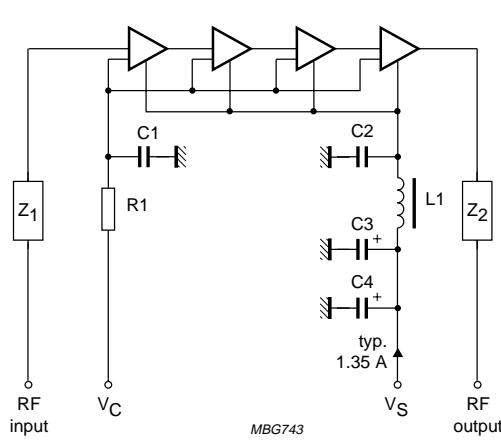
Fig.16 Test circuit.
