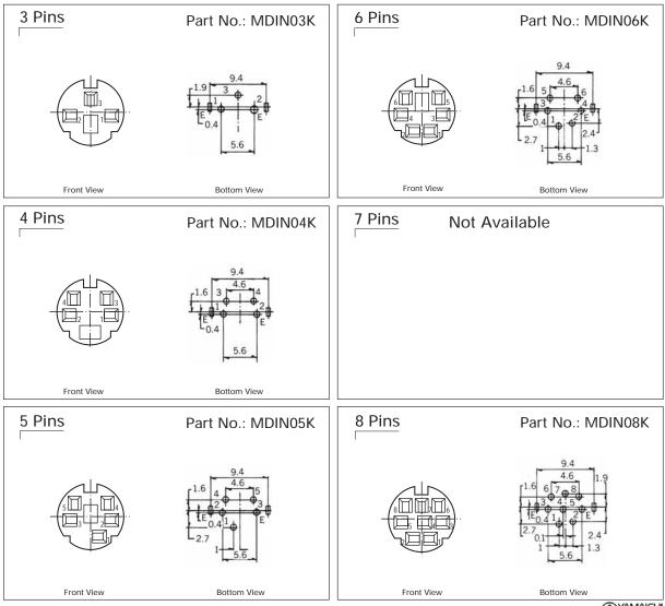
Sockets and Connectors SPECIFICATIONS AND DRAWINGS ARE SUBJECT TO ALTERATION WITHOUT PRIOR NOTICE - DIMENSIONS IN MILLIMETER **AYAMAICHI** Trading Division
