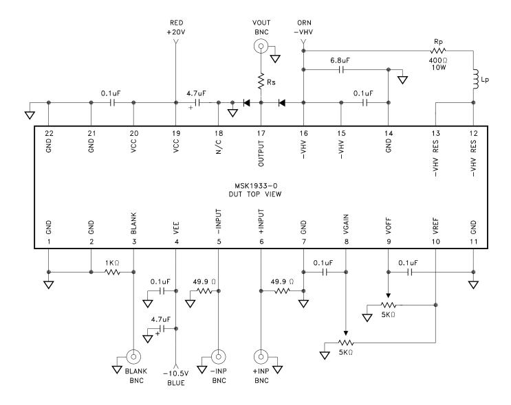
The connection circuit shown above is for the MSK 1933-0 evaluation board. The Rp and Lp are external components and must not be located near ground planes if possible. A high quality resistor such as Bradford Electronics P/N FP10-400 is required for optimum response times. Use an inductor with a high self-resonant frequency that can withstand the currents required for the application.
