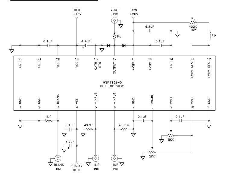
The connection circuit shown above is for the MSK 1932-0 evaluation board. The Rp and Lp are external components and must not be located near ground planes if possible. A high quality resistor such as Bradford Electronics P/N FP10-400 is required for optimum response times. Use an inductor with a high self-resonant frequency that can withstand the currents required for the application.
