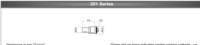
Dimensions in mm (Typical) Not to scale Green dot on base indicates centre contact cathode. -ve. Colour dot on product denotes LED colour
