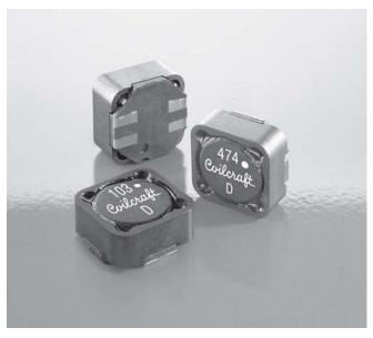
The excellent coupling coefficient ( $k \ge 0.94$ ) makes the MSD1260 series of coupled inductors ideal for use in SEPIC applications. In SEPIC topologies, the required inductance for each winding in a coupled inductor is half the value needed for two separate inductors, allowing selection of a part with lower DCR and higher current handling.
