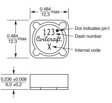
Parts manufactured prior to Sept. 2007 were marked with only the dash number.
