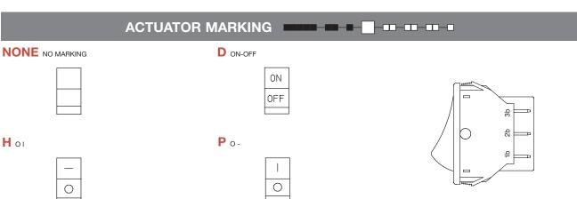
NOTE: Orientation of actuator marking and terminals. Shown in Pos. 1
