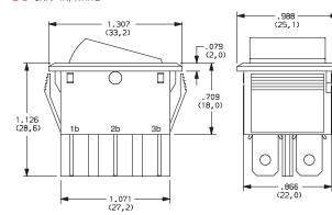
NOTE: Available with 05 termination and QA contact rating only. Shown in Pos. 1
