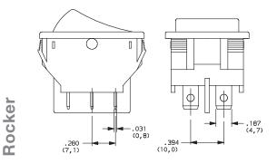
NOTE: Available with S1 & S2 mounting style and Q contact rating only. Shown in Pos. 1
