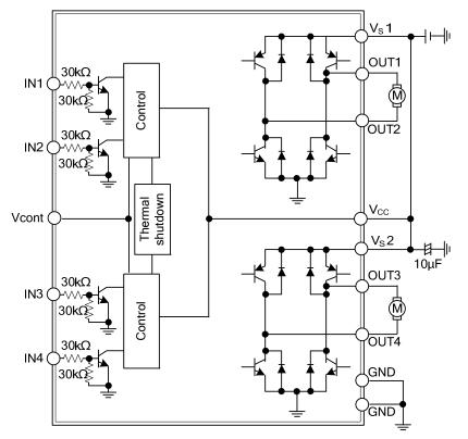
Note: There are no restrictions on the relationship of each voltage level in comparison with the others (regarding which is higher or lower), as long as the voltages applied to V<sub>CC</sub>, V<sub>S</sub>1, V<sub>S</sub>2, and IN1 through IN4 are within the limits set by the absolute maximum ratings. (Ex: V<sub>CC</sub>=3V, V<sub>S</sub>1, 2=2V, IN1 to IN4=5V)
