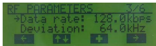
Figure 8. Menu Page: RF Parameters 3/6 (Modulation is 2GFSK)
