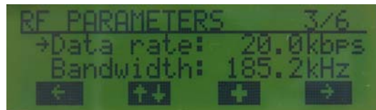
Figure 9. Menu Page: RF Parameters 3/6 (Modulation is OOK)
