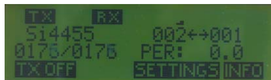
Figure 15. Running PER Test (TRx Mode)
