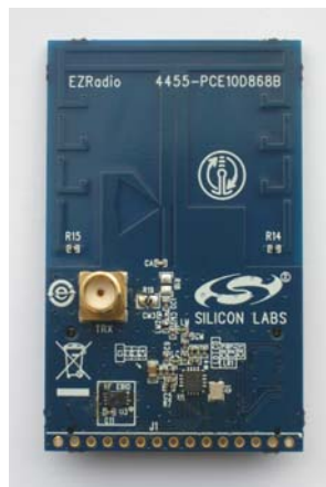
Figure 2. Si4455 RFpico Board—868 MHz (P/N 4455-PCE10D868B)
