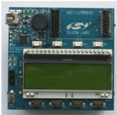
Figure 1. LCD Base Board (P/N MSC-LCDBB930-PER)
