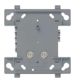
The **M500M-4-20 Analog Input Module** allows the connection of 4-20 mA output sensors to a fire alarm control panel (FACP). The module converts the sensor output to a common communication protocol that can be interpreted by the FACP for monitoring and display. There are numerous sensors available in the marketplace that communicate using a 4-20 mA output, including gas sensors, temperature sensors, air speed sensors, and more.
