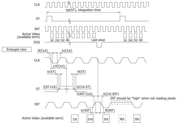
Allow CLK pulse transition from "high" to "low" only one time while ST pulse is "high". Integration time is determined by the interval between start pulses.
