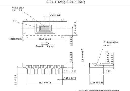
\*1: Distance from upper surface of quartz window to chip surface
