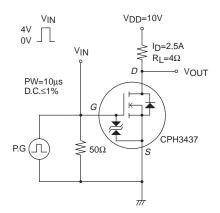
**Switching Time Test Circuit**
