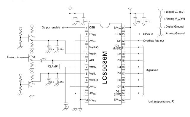
Note 1. The value of the reference resistor is about 300 Ω. When this circuit is used with (VrefH – VrefL) = 2 V, a current of 6.7 mA will flow. Use an operational amplifier or emitter follower with at least this current capacity.
