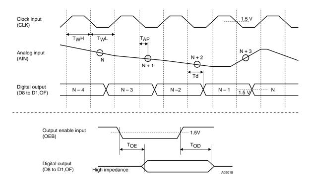
The analog signal (AIN) is acquired on the falling edge of the clock input (CLK). The acquired analog signal is converted to a digital code and is output from the digital outputs (D8 to D1, OF) on the clock falling edge delayed three clock cycles from the clock cycle in which the analog signal was acquired.
