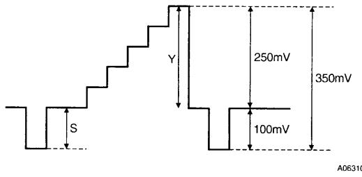
15. Measure the 4fsc (14.3 MHz) and fsc (3.58 MHz) components in the Y-OUT output with no input signal.
