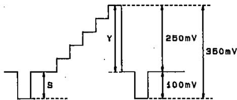
$$LS = \frac{S \text{ [mV]}}{Y \text{ [mV]}} \times 100 \text{ [%]}$$
