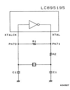
R1 = 120 k $\Omega$ R2 = 47 k $\Omega$ C1 = 30 pF For a crystal oscillator frequency of 16.9344 MHz. Alternatively: R1 = 3.3 k $\Omega$ R2 = None
