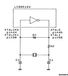
$\begin{aligned} \text{R1} &= 120 \text{ k}\Omega \\ \text{R2} &= 47 \text{ }\Omega \\ \text{C1} &= 30 \text{ pF} \end{aligned}$
