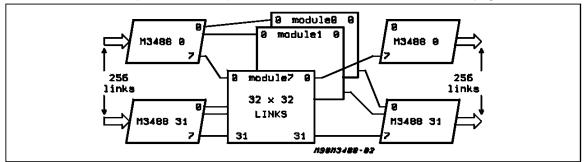
2048 PCM links network (1792 or 2048 DSM) : the 256 x 256 link network is shown above.
