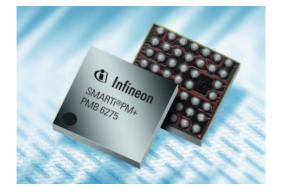
S M A R T i $^{\circ}$ P M + ( P M B 6 2 7 5) is a Quad Band EDGE/GPRS Transceiver in a groundbreaking new 3 x 3 mm $^{2}$  wafer level ball grid array package. It enables the design of Quad Band Micro EDGE RF systems in less than 100 mm $^{2}$  PCB area.
