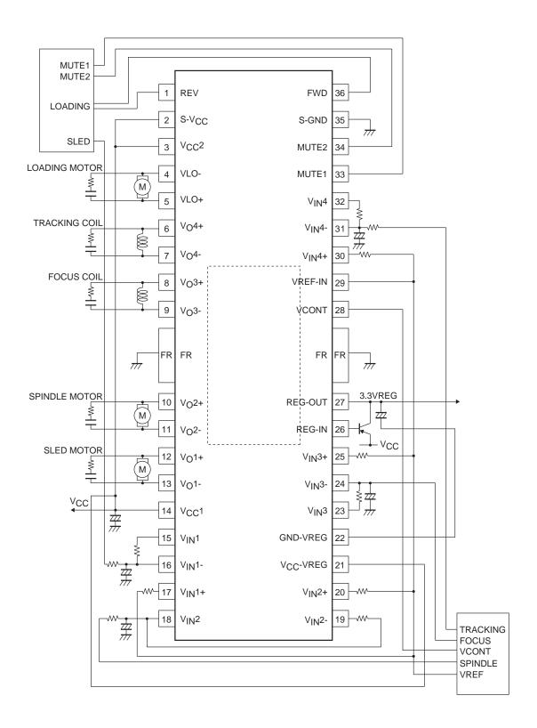
Note : Add CR between outputs or to a circuit to GND when oscillation occurs in the output (Example :  $R=2.2\Omega$ ,  $C=0.1\mu F$ ). Apply 4.5V or more to the external PNPTr emitter pin.
