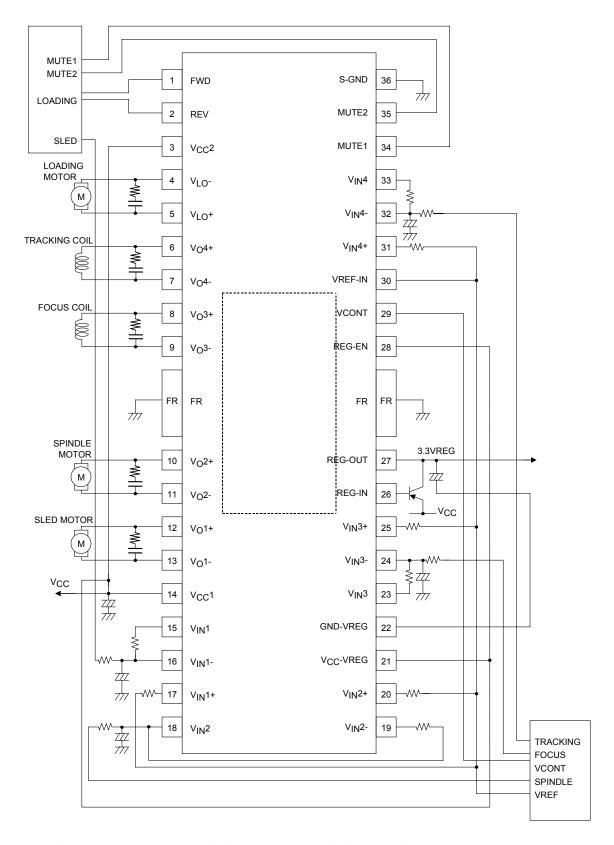
Note: Add CR between outputs or to a circuit to GND when oscillation occurs in the output. Apply 4.5V or more to the external PNPTr emitter pin.
