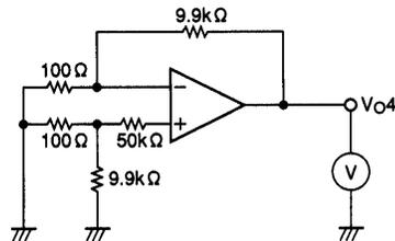
$$I_B^+ = \frac{|V_{O4} - V_{O1}|}{50k \times 100}$$
