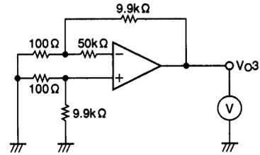
$$I_B^- = \frac{|V_{O3} - V_{O1}|}{50k \times 100}$$
