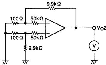
$$I_{IO} = \frac{|V_{O2} - V_{O1}|}{50k \times 100}$$
