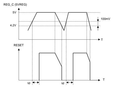
\*1: td is the delay time. It is set by an external capacitor connected between the CD pin and ground. \*2: The voltage at which RESET changes state is a typical value (voltage).
