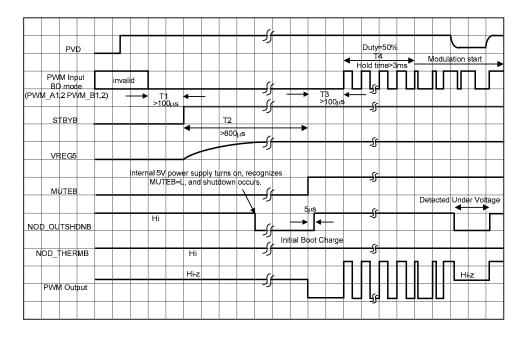
The NOD\_OUTSHDNB (Nch open drain) output signal is generated (Nch open drain output is turned on) when output is shut down (except when the overcurrent protection circuit is activated). This operating condition is established when either one of the following conditions occurs:
