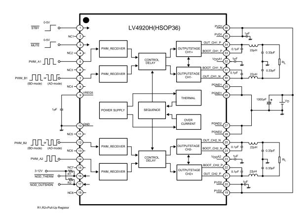
\* NOD\_THERM at pin 16 and NOD\_OUTSHDN at pin 17 are outputs of N-ch open-drain type. When CPU or other device monitors these outputs, it is necessary to connect pull-up resistors to a power supply for the CPU and other device. The pull-up resistors are not required if they are not to be used (not monitored).
