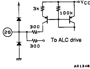
A01348 | <ul style="list-style-type: none"> <li>ALC operates at 0.65 V or higher.</li> </ul>                                                                                                                      |
