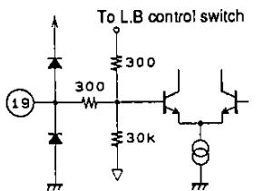
A01345   | <ul style="list-style-type: none"> <li>PVSS is turned on by the power output signal, and turned off when grounded.</li> </ul>                                                                            |
