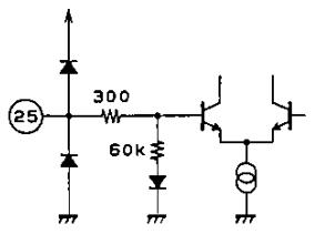
A01347 | <ul style="list-style-type: none"> <li>The low boost function is turned on when this pin is floating and turned off when it is connected to Vref.</li> </ul>                                             |
