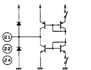
A01346  | <ul style="list-style-type: none"> <li>The power output pins</li> <li>The LA4805V drives headphones with pin 22 used as a common center. (No electrolytic capacitors are used in the output.)</li> </ul> |
