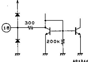
A01344   | <ul style="list-style-type: none"> <li>Smoothing pin used when PVSS is turned on and off.</li> </ul>                                                                                                     |
