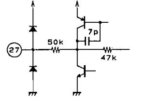
A01349 | <ul style="list-style-type: none"> <li>Low boost secondary low pass pin</li> </ul>                                                                                                                       |
