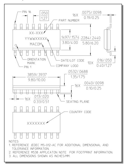
Reference Application Note M538 for lead-free solder reflow recommendations.
