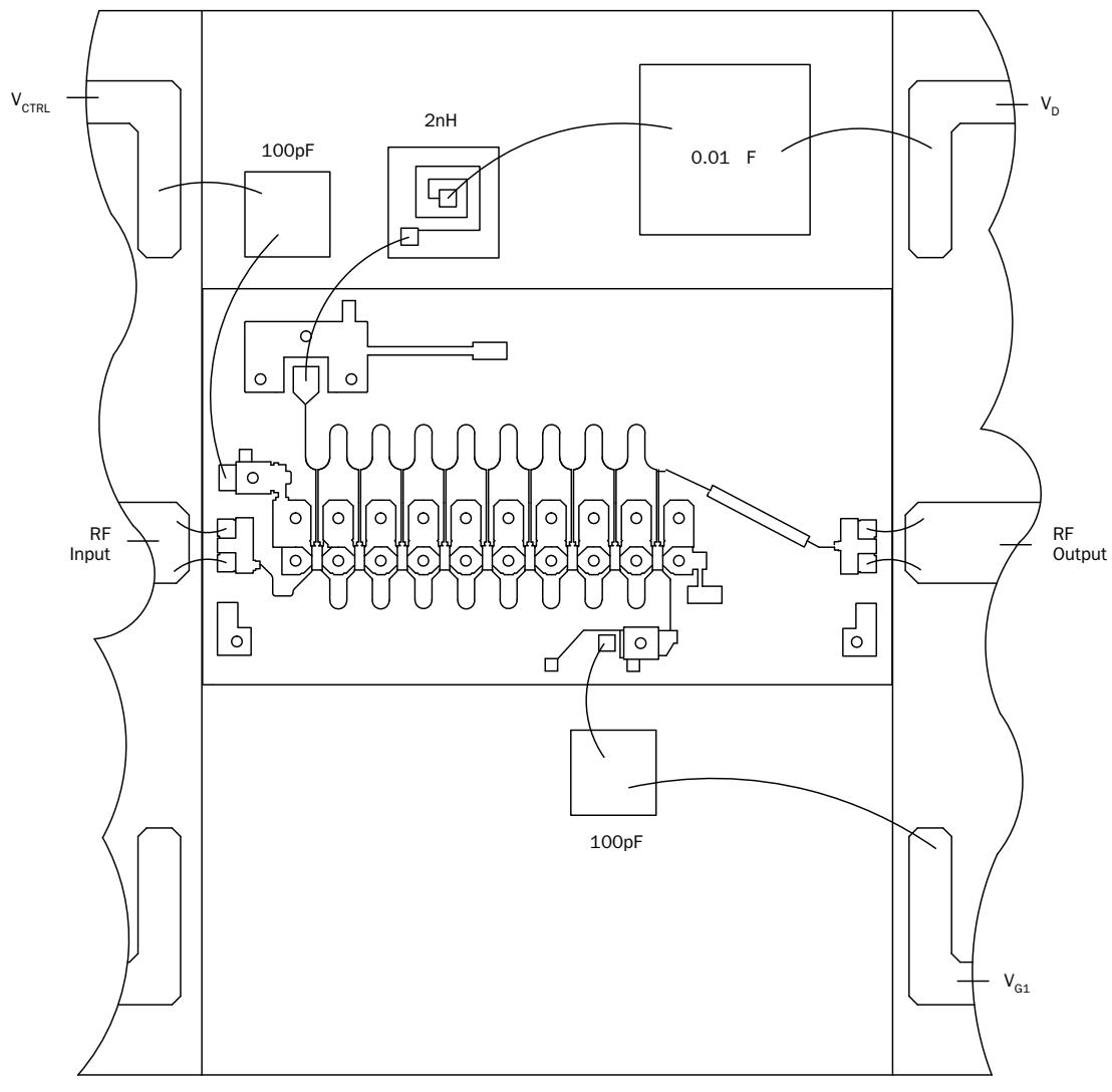
The 2-nH thin-film network coil is TI part number 3022039-1.
