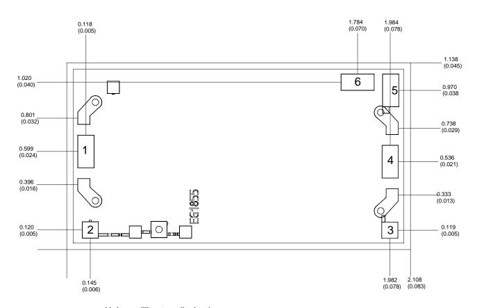
Units: millimeters (inches) Thickness: 0.100 (0.004)
