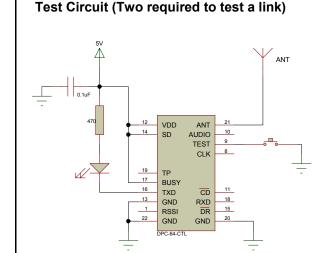
When keying the TEST switch, the DPC-64-CTL will transmit its 64 byte preset test message to the receiving DPC-64-CTL test circuit. The test transmission will continue for as long as the test button is keyed.
