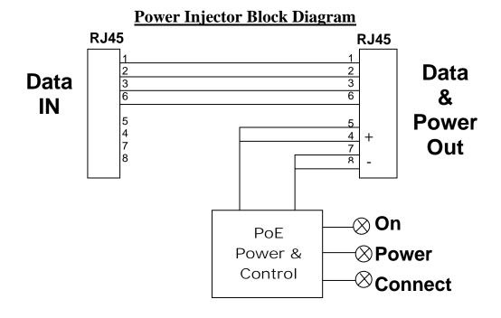
**Description of LED Functions for Power Injector**
