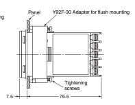
Note: 1. The recommended panel thickness is 1 to 4 mm.
