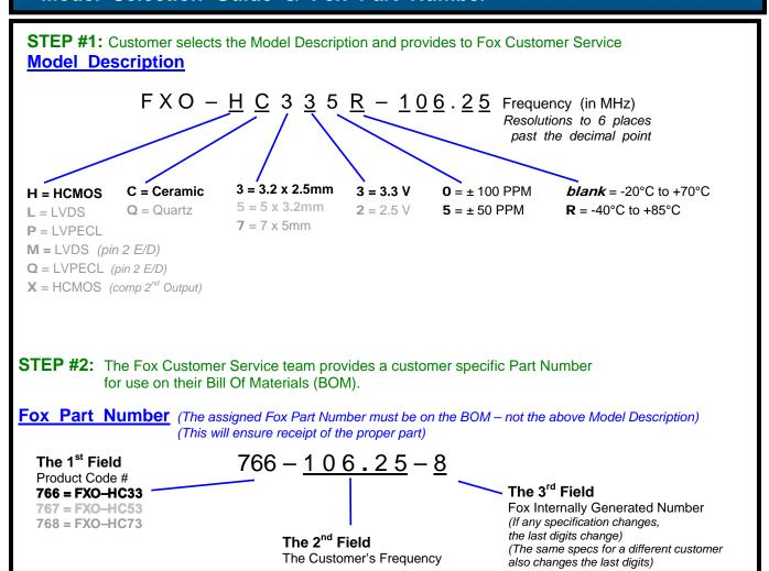
This example, FXO-HC335R-106.25 = HCMOS Output, Ceramic 3.2 x 2.5mm Package, 3.3V, ±50 PPM Stability, -40 to +85°C Temperature Range, at 106.25 MHz
