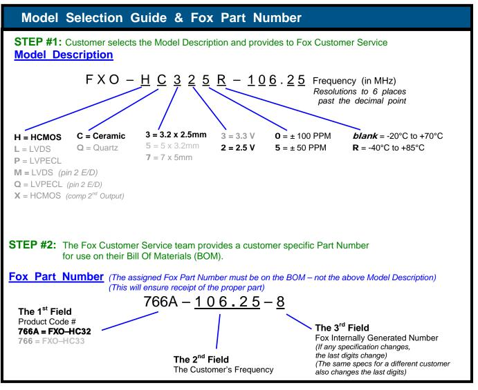
This example, FXO-HC325R-106.25 = HCMOS Output, Ceramic 3.2 x 2.5mm Package, 2.5V, ±50 PPM Stability, -40 to +85°C Temperature Range, at 106.25 MHz
