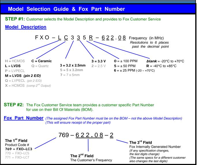
This example, FXO-LC335R-622.08 = LVDS Output, Ceramic, 3.2 x 2.5mm Package, 3.3V, ±50 PPM Stability, -40 to +85°C Temperature Range, at 622.08 MHz
