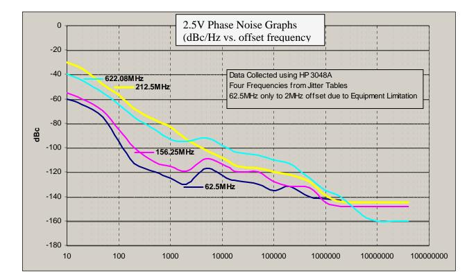
Jitter is frequency dependent. Below are typical values at select frequencies.
