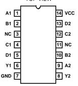
14 LEAD CERAMIC METAL SEAL FLATPACK PACKAGE (FLATPACK) MIL-STD-183S CDFP3-F14 TOP VIEW
