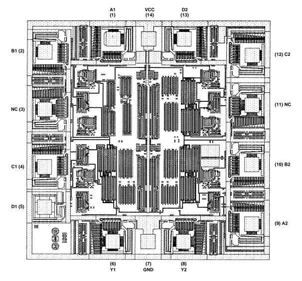
NOTE: The die diagram is a generic plot from a similar HCS device. It is intended to indicate approximate die size and bond pad location. The mask series for the HCTS20 is TA14426A.
